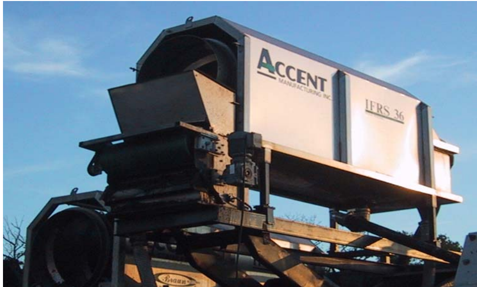
Figure 9 – Accent Rotary Separator for Solids Removal at Ripp Dairy Valley Farm Demonstration
